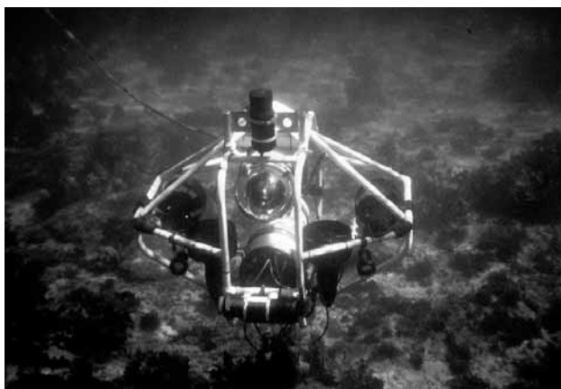
Figure 10.6 Underwater vehicle Oberon, developed at the University of Sydney. Image courtesy of Stefan Williams and Hugh Durrant-Whyte, Australian Centre for Field Robotics.
