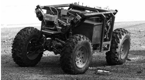
Figure 11.4 The Groundhog robot is a 1,500 pound custom-built vehicle equipped with onboard computing, laser range sensing, gas and sinkage sensors, and video recording equipment. The robot has been built to map abandoned mines.
