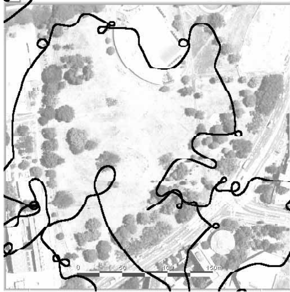
Figure 12.14 The testing environment: A 350 meter by 350 meter patch in Victoria Park in Sydney. Overlaid is the integrated path from odometry readings. Data and aerial image courtesy of José Guivant and Eduardo Nebot, Australian Centre for Field Robotics; results courtesy of Michael Montemerlo, Stanford University.
